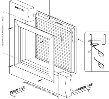
Adjustable Fusible Link Louvers are recommended for use in rooms where ventilation is needed and at the same time isolating the room whenever fire is present. When louver is exposed to heat at 165°F, the fusible link trips and the spring loaded louver blades shut to form an air tight fire and smoke seal.
